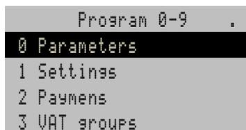
The display reading shows that ECR is in programming mode and awaits sub-mode selection.
