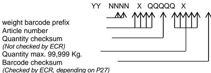
**SALES WITH QUANTITY USING ELECTRONIC SCALE**
